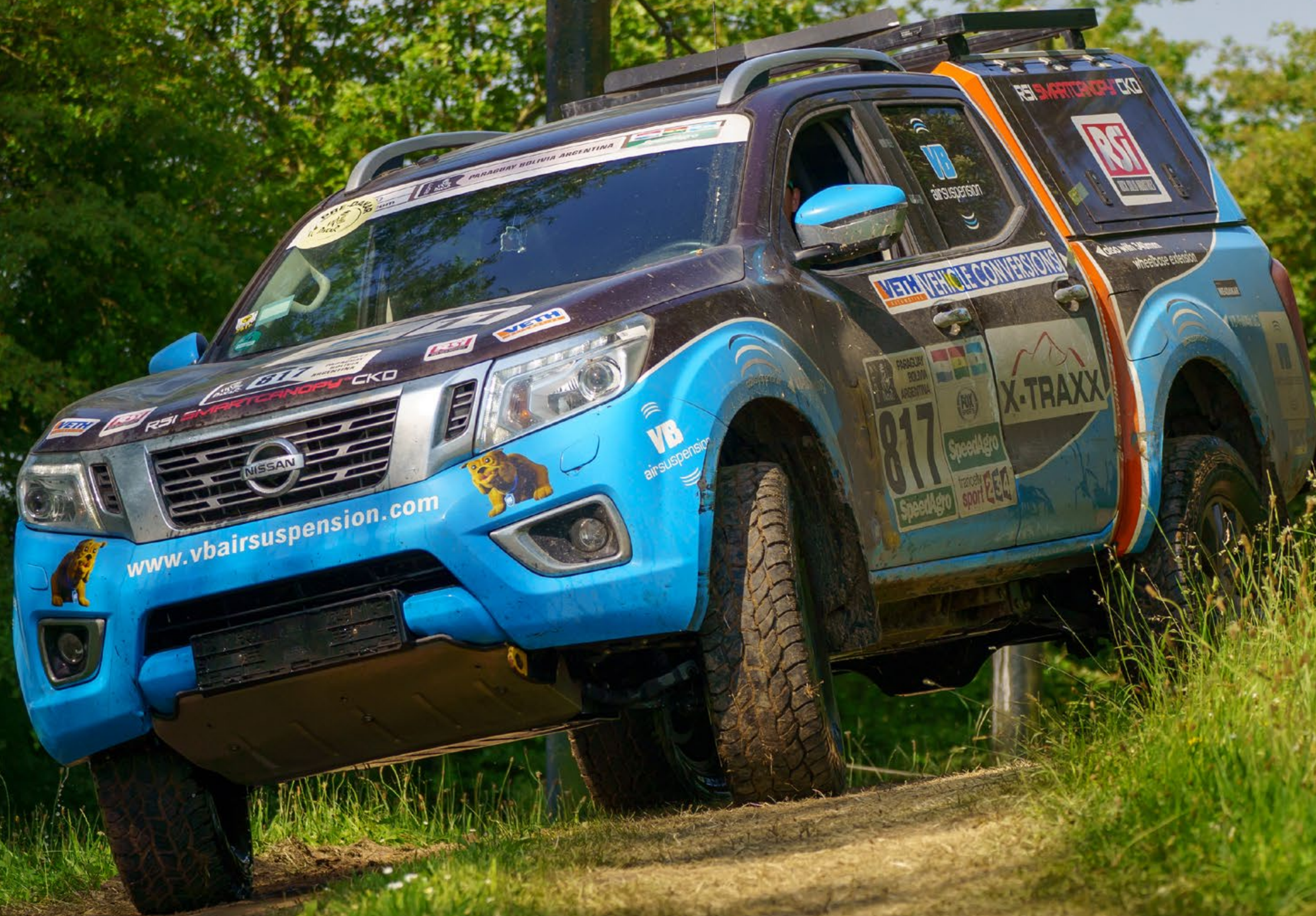
PHOTOGRAPH This VB-Airsuspension Nissan Navara with a VB-FullAir 2C air suspension system has already shown what it can do at the 'Le Dakar' in South America and the 'Morocco Desert Challenge' in Morocco.
